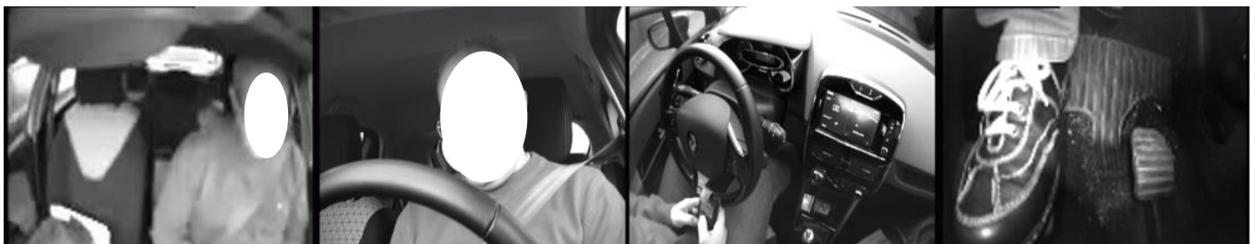
Fig. 1: Example of the four different views. From left to right, cockpit, driver, top view and pedals cameras.
