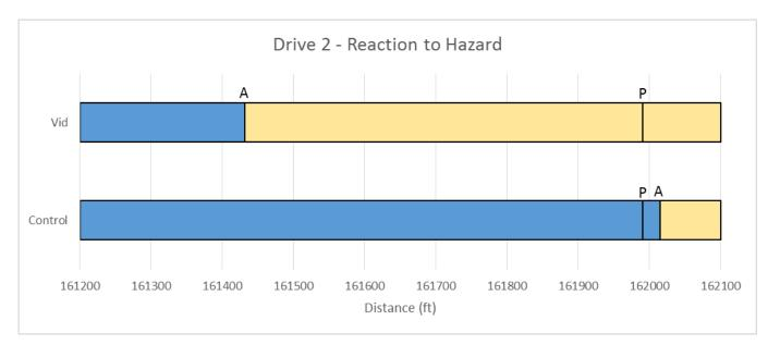
Fig. 4. Mean distance at which drivers lifted their foot from the accelerator in response to a potential hazard (A = Participant's foot lifts from accelerator, P = Pedestrian begins walking)
