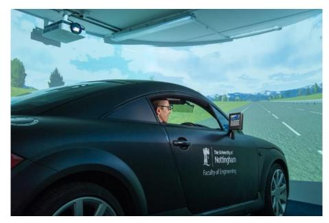
Fig. 1. Medium-fidelity driving simulator showing motorway scenario used during study.
