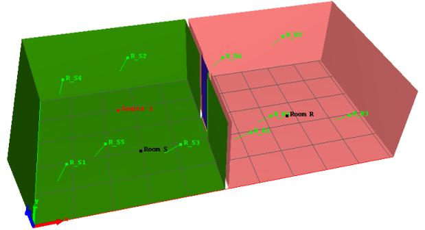
Figure 1: Coupled rooms geometry. See table 4 for details.
